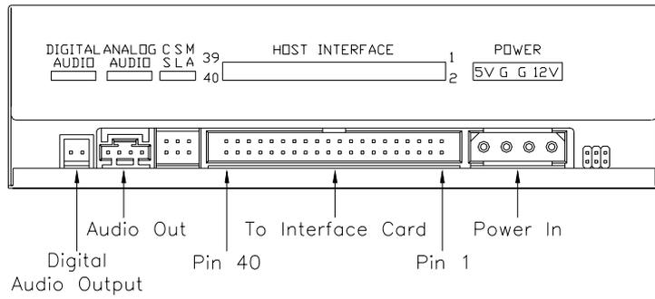
☞ *The red-edge of the IDE Cable must be connected to Pin 1 on the CD-ReWritable drive.*
